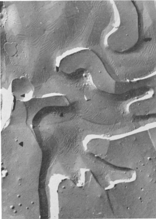
Figure 5 Dendritic cavity profile with rounded surface and curved terraces. Strained at 850^{\circ}\text{C} and 1.6 \times 10^{-1} \text{ h}^{-1} ( \times 4000 ).
