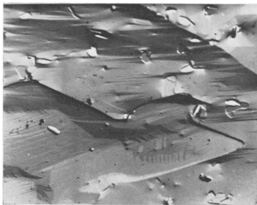
Figure 9 Cavity showing terracing and preferred growth direction with "gouge" markings on the uncavitated grain-boundary surface, strained to 6% extension at 700^\circ\text{C} and 5\% \cdot 10^{-4} \text{h}^{-1} ( \times 4400 ).
